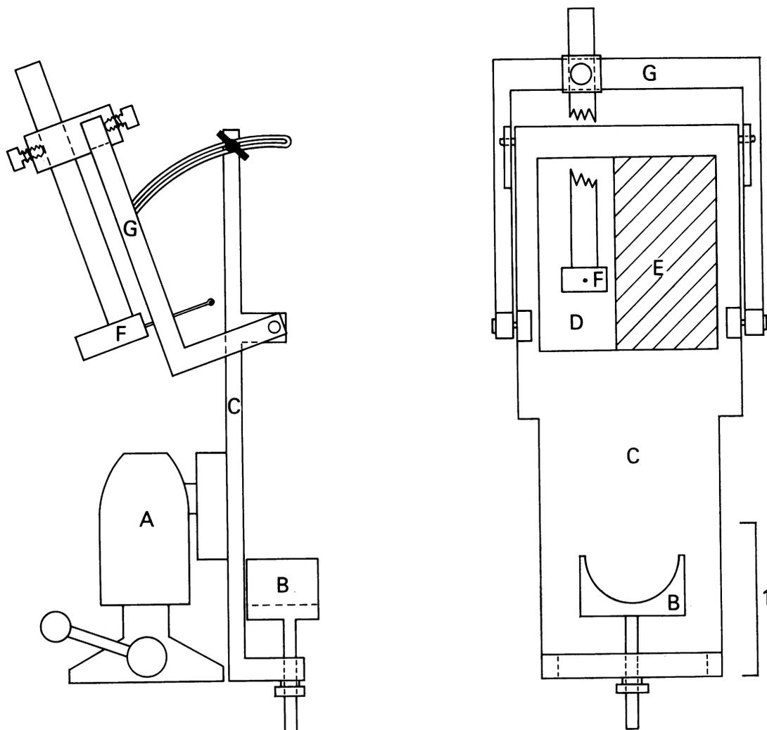
FIG. 1. Adjustable foot holder for EHB twitch experiments, viewed from the side (left) and the front (right). In the latter view the U-bar has been rotated into a plane parallel with that of the base-plate (C). For description of parts and technique of use, see text.
