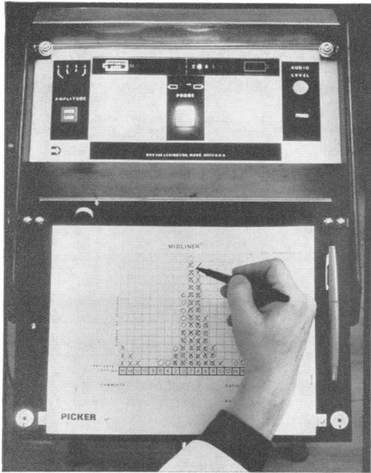
FIG. 1 Investigation with the Midliner. Note lack of oscilloscope. Readings appear on digital scale.
