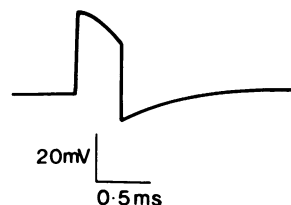
Fig 5 Voltage waveform of a single pulse recorded across a 10 ohm resistor in series with electrode. The vertical section of the waveform indicates the voltage across the resistor while peak current is flowing, in this case about 18 mV, indicating a peak current of 1.8 mA.
