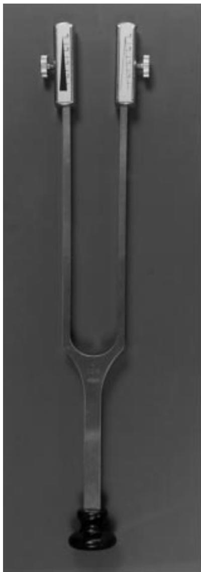
The Rydel-Seiffer (RS) tuning fork (Martin, Tuttingen, Germany). Note the triangle and arbitrary scale from 0 (minimum score) to 8 (maximum score) imprinted on the weights of the two arms that allow quantitative vibration assessment.<sup>17</sup>
