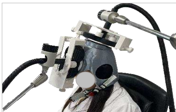
Figure S4-1. Custom-made 3D-printed helmet
